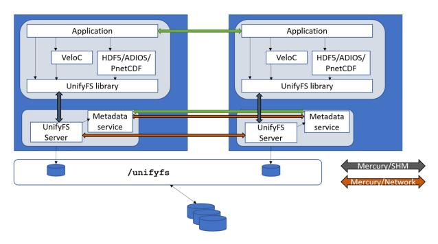
This section provides a high level design of UnifyFS. UnifyFS presents a shared namespace (e.g., /unifyfs as a mount point) to all compute nodes in a job allocation. There are two main components of UnifyFS: the UnifyFS library and the UnifyFS server.
